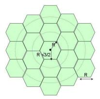
Carrier to Interference Ratio (CIR) and cell capacity
