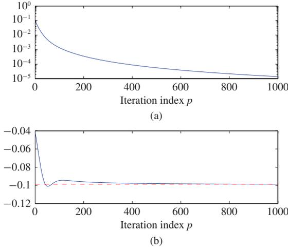
Fig. 1. Example of sublinear convergence speed. (a) Decrease of the objective function  $J$  ( $\eta = 1$ ). (b)  $1/\|\mathbf{H}^{(p)} - \mathbf{H}\|_F - 1/\|\mathbf{H}^{(p+1)} - \mathbf{H}\|_F$  ( $\eta = 1$ ).
