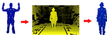
Figure 5: Our Kinect calibration pose (left), applied to the pre-recorded depth map for Anne-c1-t1 (centre), giving a skeletal overlay (right).
