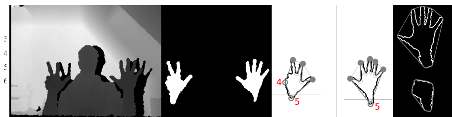
Fig. 3: left: depth map; middle: isolated hands; right: fingertip detection: hand contour (black), simplified hand contour (gray), fingertips (gray circles), vertices marked with 4 or 5 were removed from the list of fingertips in the corresponding processing step
