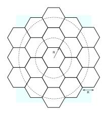
Figure 1. Cluster of a hexagonal network centrally controlled by the DSA algorithm.
