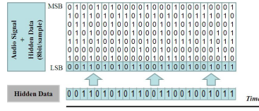
Figure 3: LSB in 8 bits per sample signal is overwritten by one bit of the hidden data.
