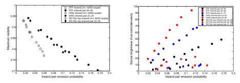
Using a laser diode (DFB) operating at 779 nm, we focus our laser beam into a PPLN crystal to generate photon pairs. True coincidences have been observed only when delaying the detection on one of the two channels. Depending on the filters, the delay can either be the same (DG) or exhibit a large variation between all channel pairs (AWG and DTF).
