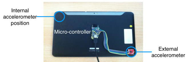
Figure 3. Test prototype with an external accelerometer.
