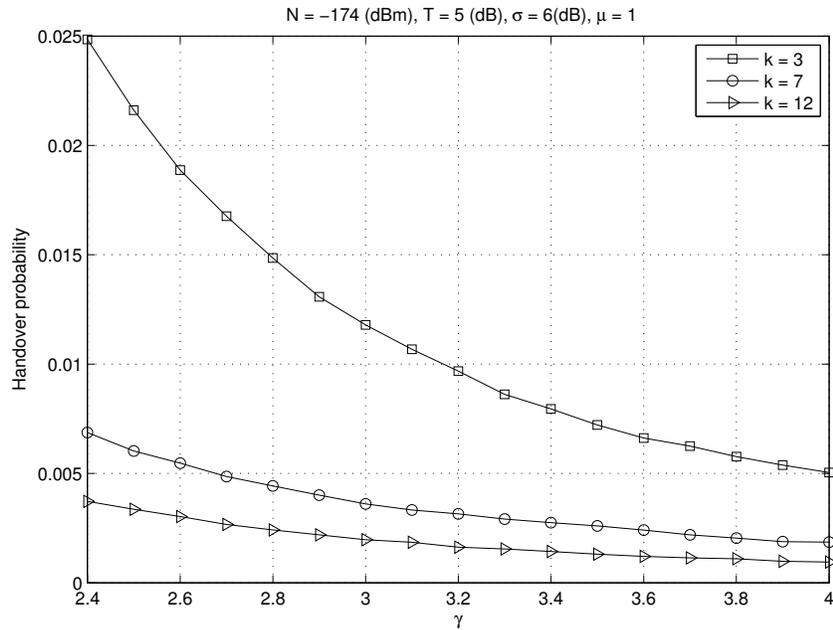
FIGURE 5. Handover probability vs path loss exponent  $\gamma$ , Poisson model,  $n = 3$
