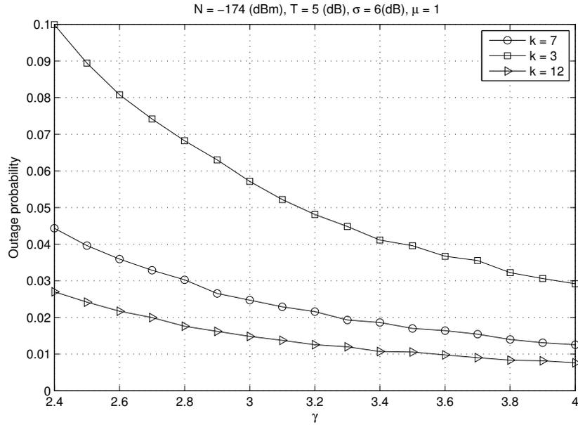
FIGURE 4. Outage probability vs path loss exponent  $\gamma$ , Poisson model
