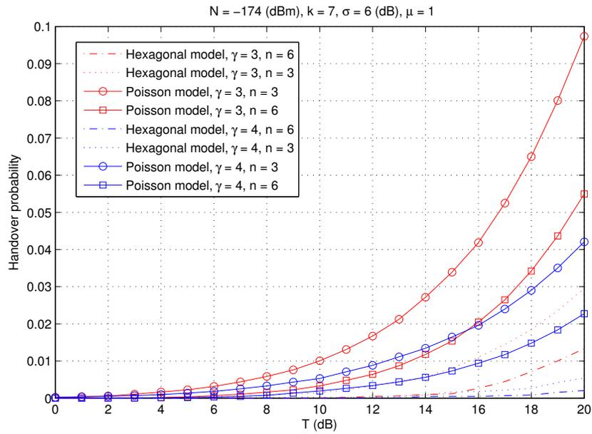
FIGURE 3. Handover probability vs SINR threshold
