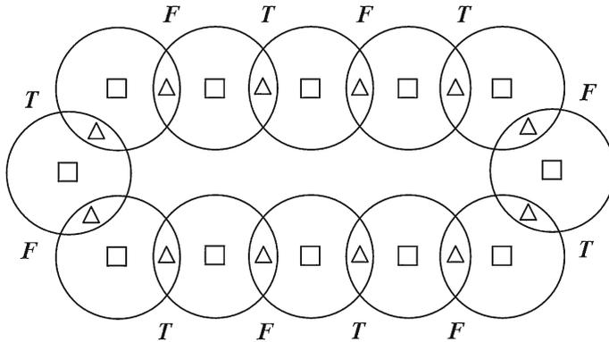
**Fig. 2** A circuit for Boolean variable  $x_i$  or  $y_j$  in the reduction. Squares indicate clients, triangles are sites for stations, T = True, F = False
