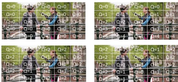
Figure 1 – Examples of priority assignment (from left to right and top to bottom): uniform, top-bottom row-based, center-based priority assignment, middle-column based priority assignment
