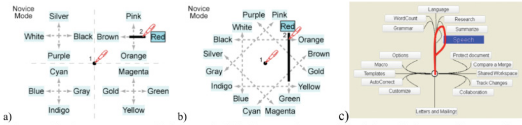
Fig. 16. (a) Zone menus [Zhao et al. 2006], extend menu breadth to 32 items. The user first taps to specify the menu origin. This action virtually splits the screen into four spatial areas corresponding to a different breadth-4 marking menu that the user activates in the usual way. (b) Polygon menus work in a similar way except that the items are the vertices of a N-sided polygon to contain up to 16 items. (c) Flower menus [Bailey et al. 2008] extend menu breadth to 56 items by combining orientation and four levels of curvature.
