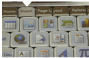
Fig. 22. Command-hotkey mapping displayed on the keyboard. The TDK Keyboard [Block et al. 2010]. Icons are dynamically displayed on the corresponding hotkey.
