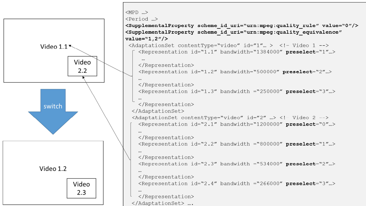
Figure 3: MPD example with the proposed quality control descriptors and new @preselect attribute
