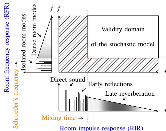
Fig. 1. Time-frequency profile of reverberation (adapted from [8] and [9]).
