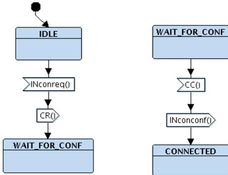
Figure 12: Protocol Machine – On Board Side
