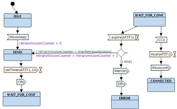
Figure 24: New Protocol Machine On the Ground Side
