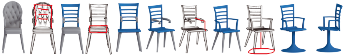
Figure 17: Overview of the workflow induced by Sketch-to-Design [XXM*13]. The user begins with an arbitrary shape (in gray) and can sketch (in red) the parts he wants to put in the final model. Parts found in the database are in blue, and symmetries are taken into account (e.g. the arms of the chair). It is possible to change the view for a better sketching experience.
