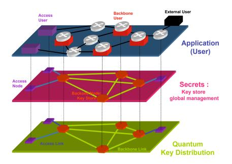
Figure 1: Logical Architecture for the QKD network.
