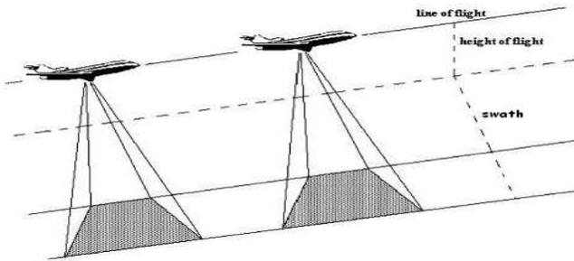
Fig. 1. Acquisition geometry by an airborne radar.
