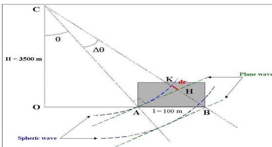
Fig. 2. Airborne radar emitted plane and spheric waves illuminating a scene with a characteristic dimension  $l$ .
