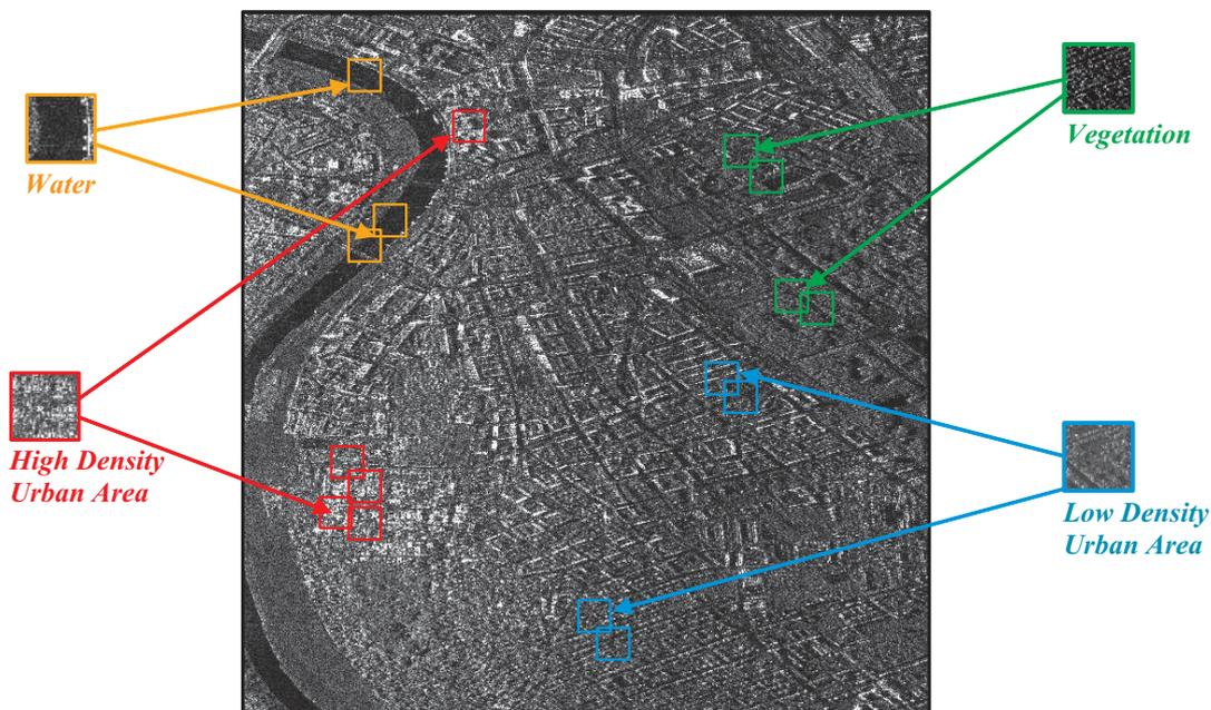
Figure 2. HR SAR image over the city of Dresden in Germany and samples of each class.
