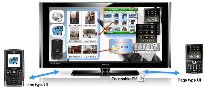
Fig. 1. Example of aggregation of and communication between two widgets coming from two different devices on a DTV. Each widget shows the file system of its corresponding device. A picture is transferred from one device to the other by a drag and drop operation on the DTV.
