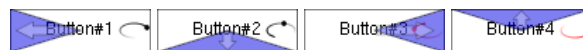
Figure 5. Semi-translucent triangle quarters indicating the top four motion matches. These quarters become a four-item pie menu when the user transitions to the next mode (by clicking).
