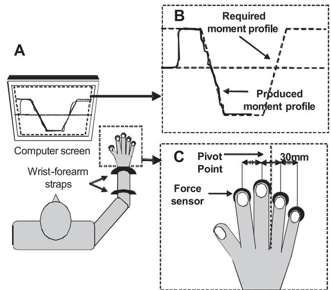
Fig. 1. A: schematic illustration of the experimental setup. B: the experimental task shown on the computer screen. C: finger and force sensor configuration.
