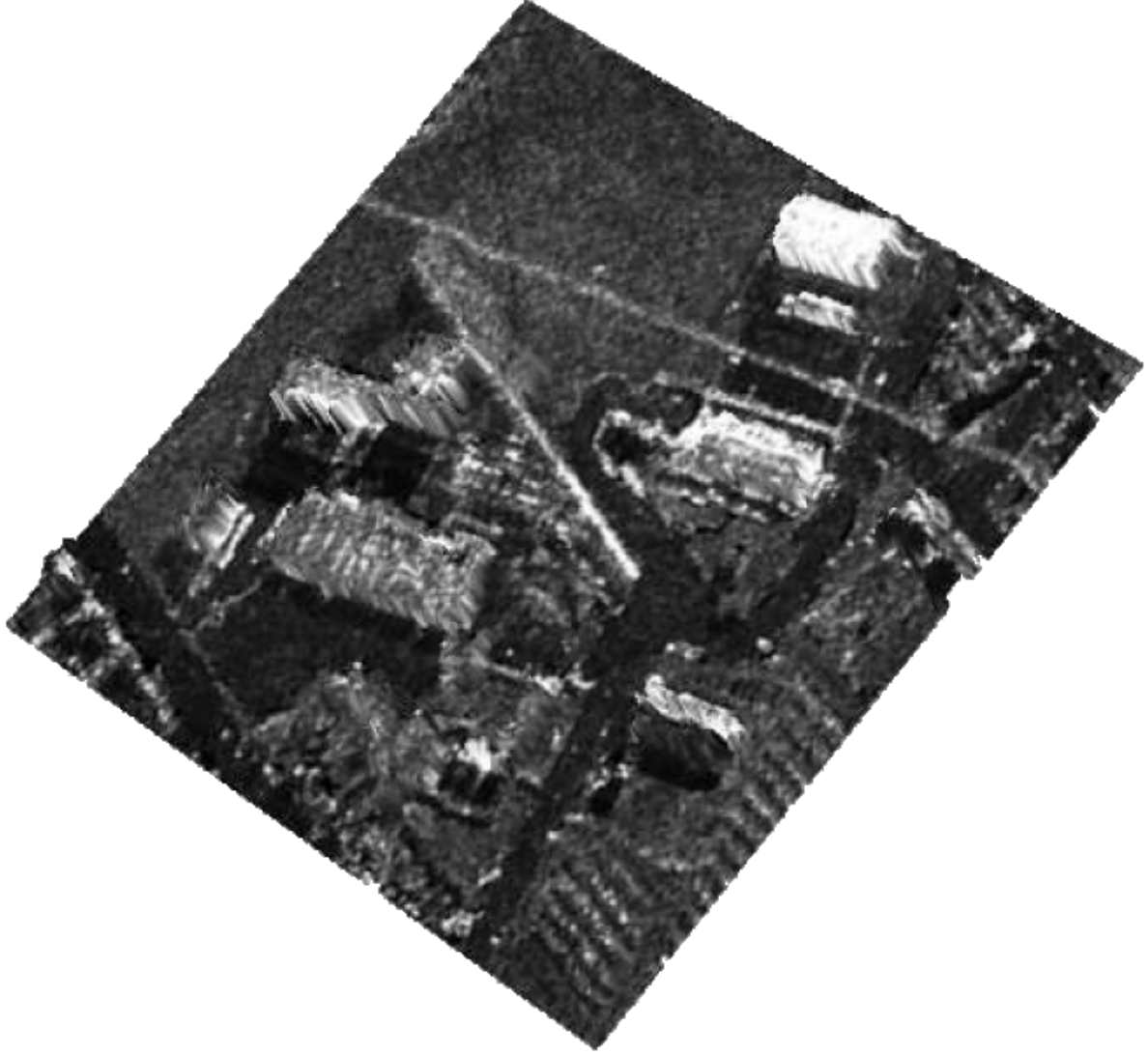
Fig. 3. 3D view of the amplitude superimposed on the elevation derived from the regularized phase.
