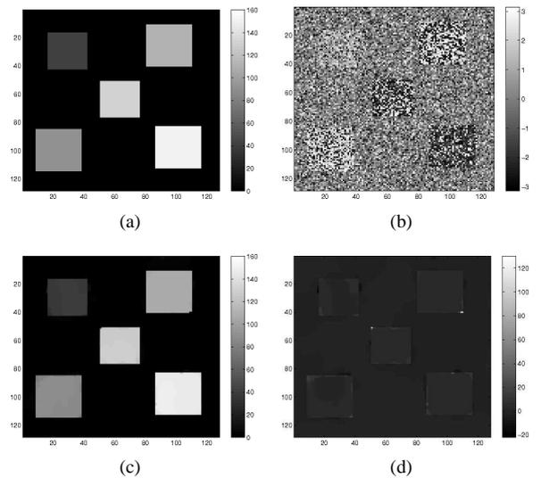
Fig. 2. MCPU results based on  $TV$  model and Ishikawa exact optimization algorithm. (a) Original urban profile, (b) Noisy interferogram at  $5GHz$  with  $\gamma = 0.5$ , (c) Reconstructed profile, (d) Difference between ground truth and estimated profiles.
