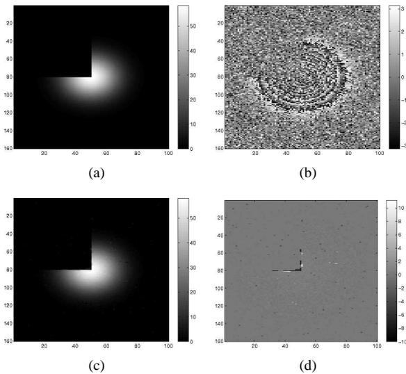
Fig. 3. *MCPU* results based on *TV* model and Ishikawa exact optimization algorithm. (a) Original Gaussian profile, (b) Noisy interferogram at  $5GHz$  with  $\gamma = 0.5$ , (c) Reconstructed profile by our approach, (d) Difference between ground truth and estimated profiles by our method
