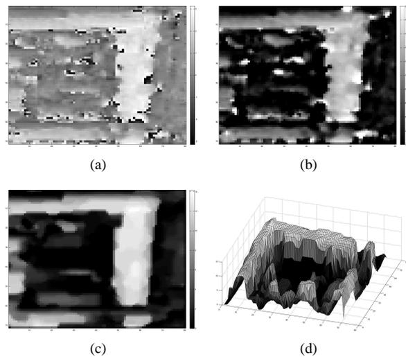
Fig. 4. 3D reconstruction of real data. (a) Noisy interferogram (smallest baseline), (b) reconstruction with branch-cut algorithm, (c) reconstruction with the proposed multichannel approach, (d) 3D view of the reconstruction with the proposed multichannel approach.
