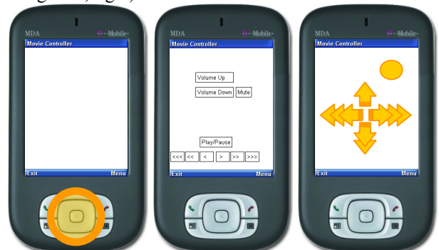
Figure 3 The three interaction methods on the mobile phone: Hardware buttons, software buttons, and gestures on the touch-sensitive display
