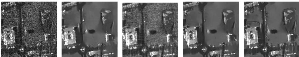
(d) Noisy image  $y_{t_3}$  (1-look). From left to right: noisy image, PPB result, 3D-ANF result, T-PPB result and 2S-PPB result.
