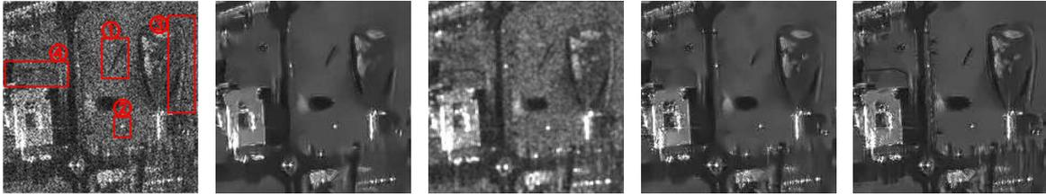
(a) Image  $y_{t_1}$  (1-look). From left to right: noisy image, PPB result, 3D-ANF result, T-PPB result and 2S-PPB result.
