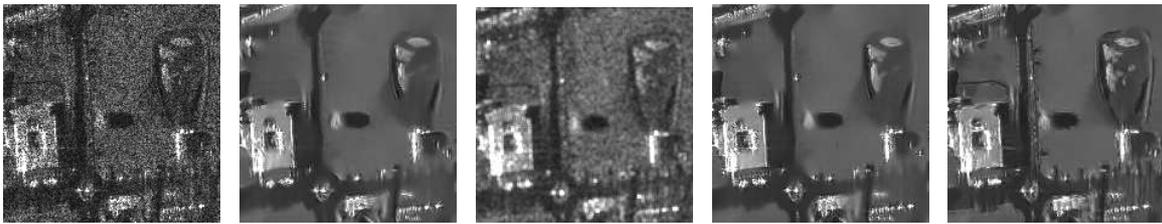
(c) Noisy image  $y_{t_2}$  (1-look). From left to right: noisy image, PPB result, 3D-ANF result, T-PPB result and 2S-PPB result.
