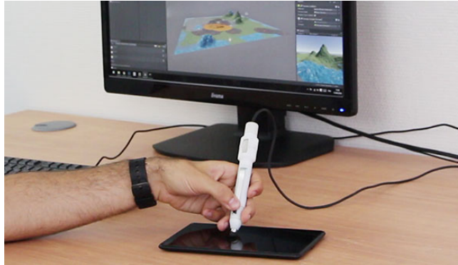
Figure 5: VersaPen in use with a 3D sculpting tool ( Unity3D ). Different input methods are combined to improve workflow and adapt input methods for specific tasks.
